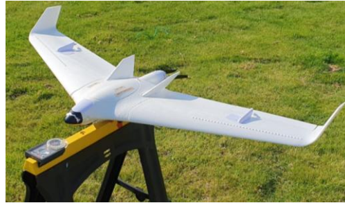
Figure 1. PAD on its stand for final system tests prior to a hand launch for flight.
