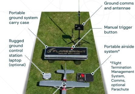
Fitted flight termination recovery system (parachute optional)
